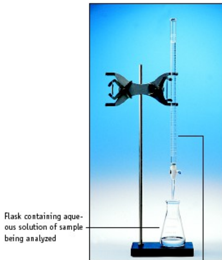
(a) 50-mL buret containing aqueous NaOH of accurately known concentration
